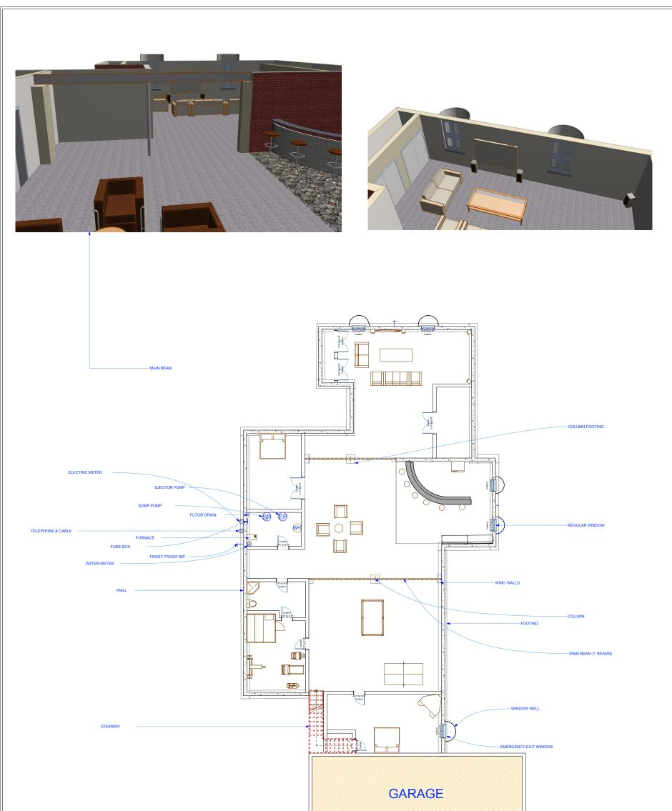
BASEMENT FLOOR - 4", W/6 MIL MOISTURE BARRIER 1/4" PEA GRAVEL GARAGE FLOOR - 4" POURED CONCRETE SLAB WITH TO-TO WWM 6X6, 1/4" PEA GRAVEL
